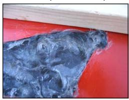
In about four hours, this will give you a solid piece of fiberglass. Then, peel back the foam board from fiberglass.
